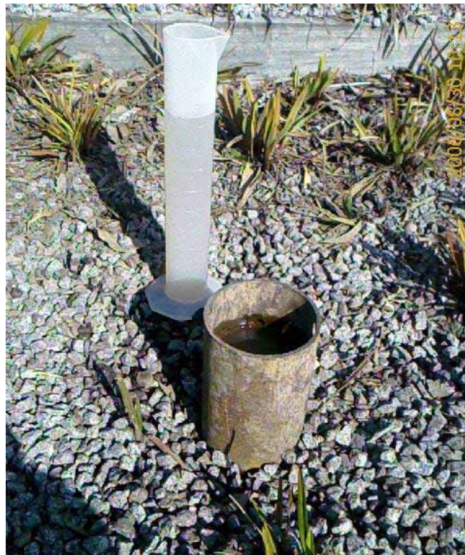
Figure 2-2 Infiltration rate test rig installed on site
