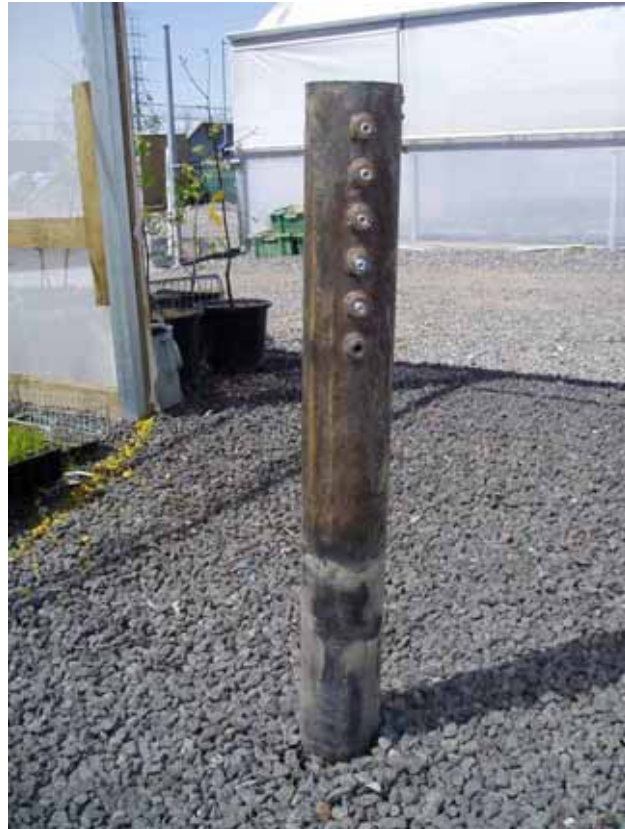
Figure 2-1 Infiltration rate test rig
